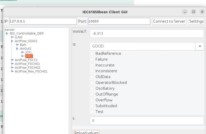
The screenshot shows the IEC61850bean Client GUI. The IP address is 127.0.0.1 and the port is 10003. The 'mxVal.f:' field displays the value -8.313. The 'q:' dropdown is set to 'GOOD'. A list of checkboxes for error states is visible, including BadReference, Failure, Inaccurate, Inconsistent,OldData, OperatorBlocked, Oscillatory, OutOfRange, Overflow, Substituted, and Test. A 'Reload values' button is at the bottom.
